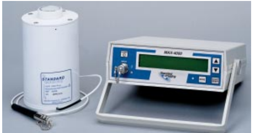
HDR 1000 Plus Well Chamber and the MAX 4000 Electrometer.
