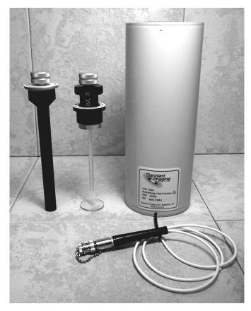
From left to right, the X-Ray Contamination Test Tool (REF 70042), Source Holder for  ${}^{90}$ Sr/ ${}^{90}$ Y (REF 70036) and the IVB Well Chamber (REF 90009)
