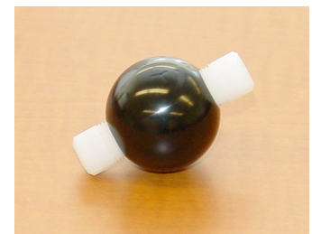
Figure 2 – Sealing ball for use with Ø12.7 mm stem.
