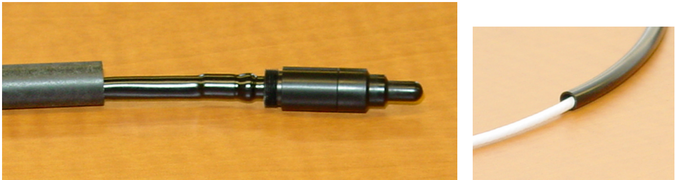
Figure 1 – Standard configuration of (vented) Exradin Thimble Chamber and open end of black tubing.
